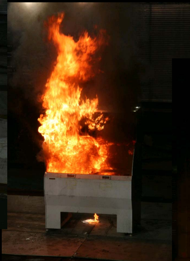
Polypropylene hood fire FM Global Research Center – November 2004
